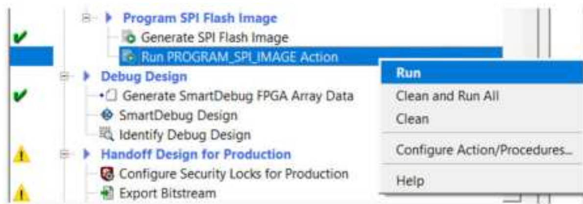
Figure 8-76. SPI Flash Programming with PolarFire Device
