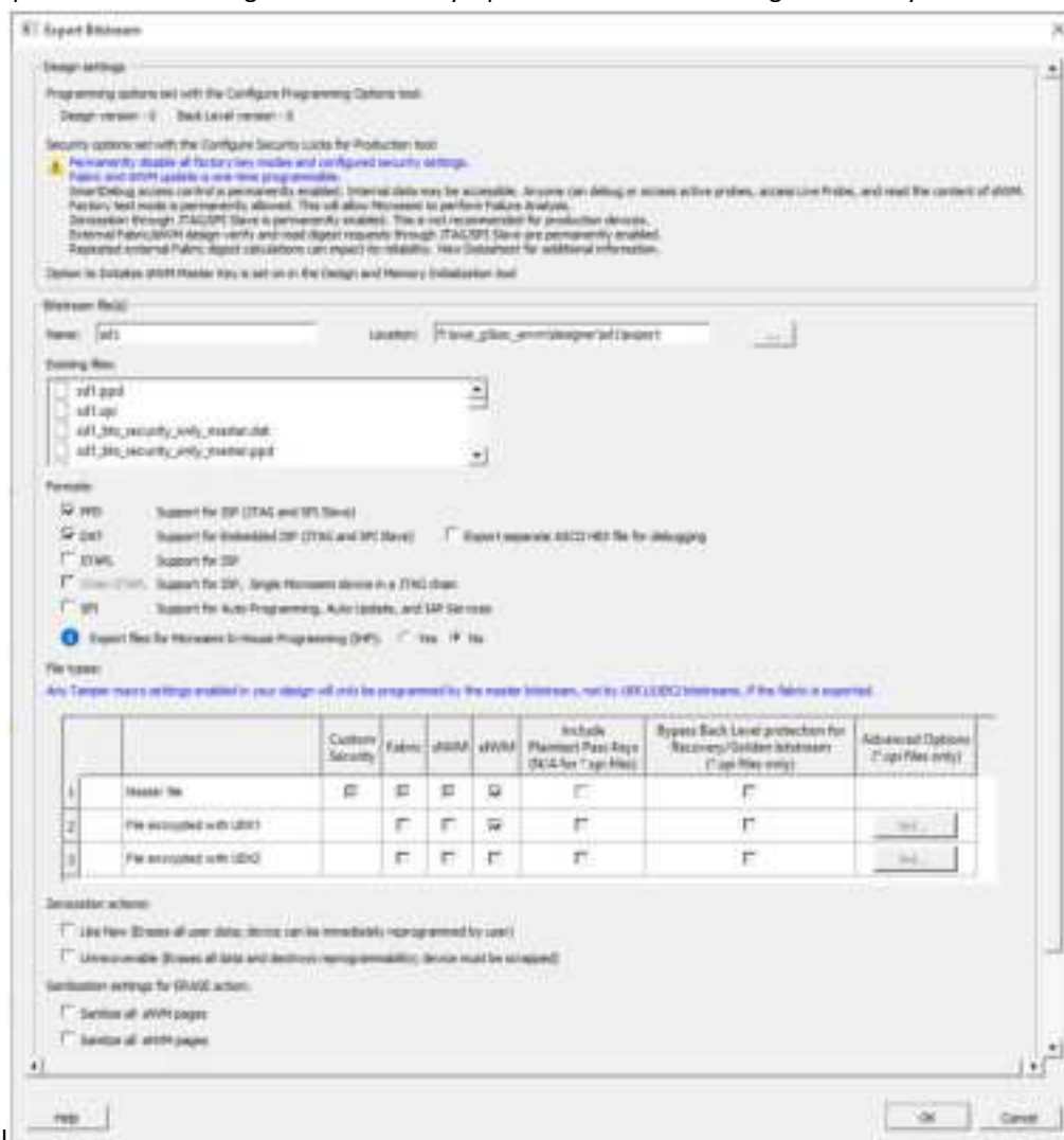
Figure 10-14. Export Bitstream Dialog Box with Security Options Set with the Configure Security Locks for
