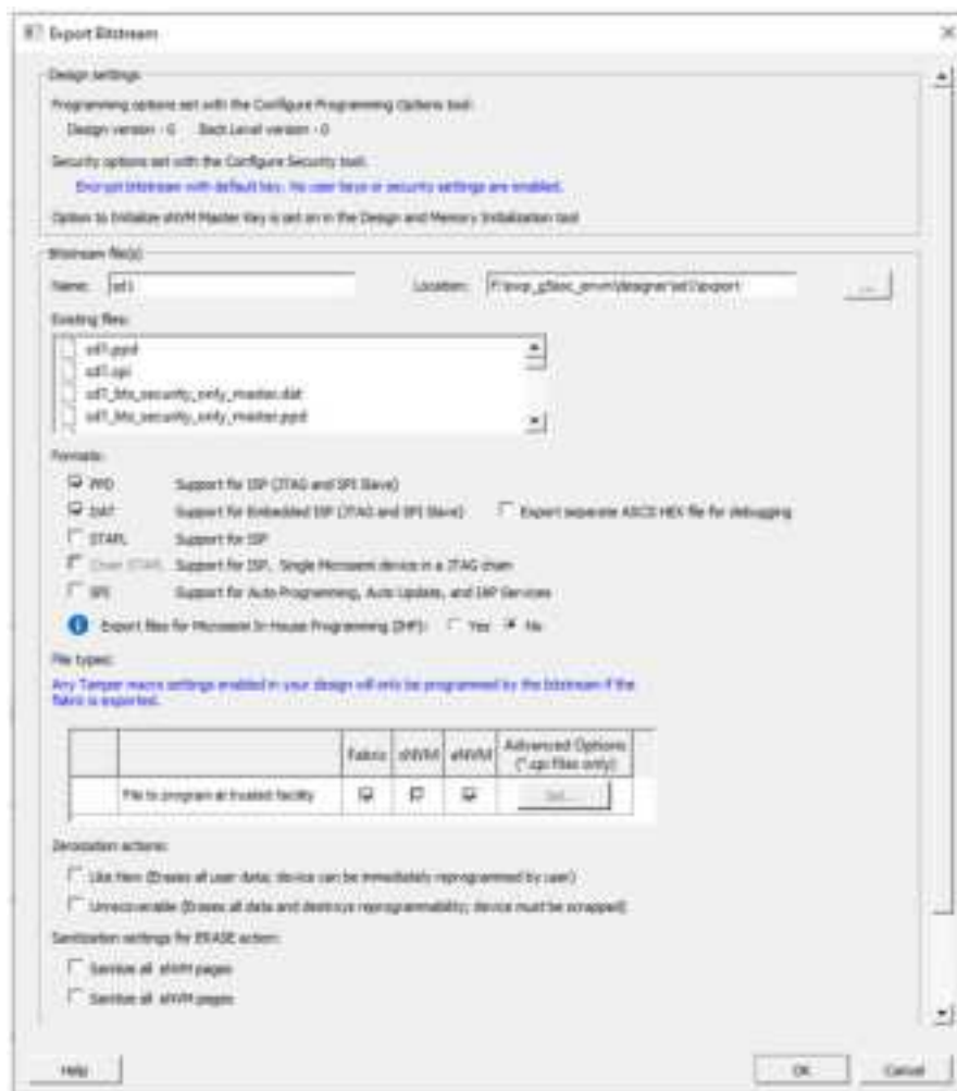
Figure 10-4. Export Bitstream Encrypted with Default Key Dialog Box (PolarFire SoC)
