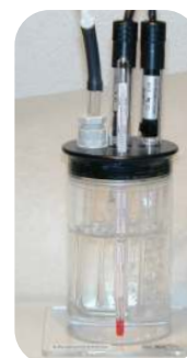
CAL300 with microensors and bubbling with air.
