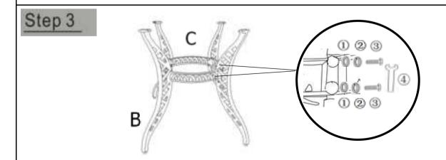
Repeat Step 2, attaching the remaining 3 Legs to the Central Round Support Ring(C).
