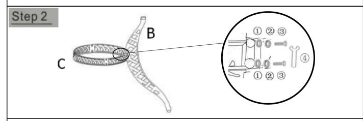
Loosely attach the Central Round Support Ring(C) to Table Leg(B) using Washers(1), Spring Washers(2), and Hex Bolts(3) with the Spanner(4). **Do not fully tighten Bolts.**
