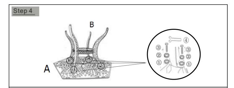
Lay the Table Top(A), top facedown, onto a flat, soft, clean surface. Loosely attach the Table Legs(B) to the the Table Top(A) using Washers(1), Spring Washers(2), and Hex Bolts(3) with the Spanner(4).
