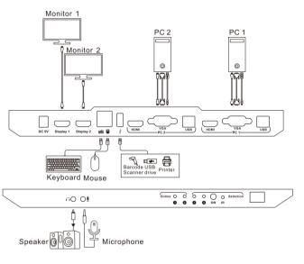
Note: Both HDMI and VGA cables should be connected to PC, if only connect HDMI or VGA cable, then the dual monitor function would not work properly.
