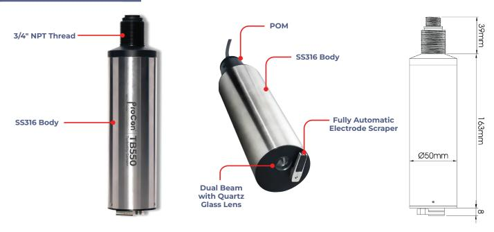
The turbidity sensor is based on infrared scattered light technology. The infrared light emitted by the light source will be scattered when it passes through the sample under test during transmission. The intensity of the scattered light is directly proportional to the turbidity.
