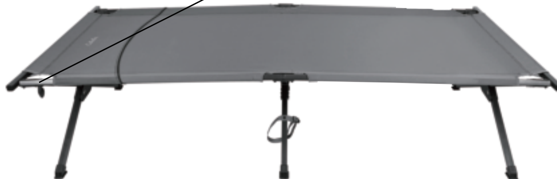
Step 5 Slide the other end bar through the pocket at the head of the cot. Locate the lever arm and make sure that it is in the unlock position. Connect end bar to the cot frame by placing the end bar notches over the plastic buttons on the cot frame. Rotate the lever arm to the lock position to lock the end bar in place.
