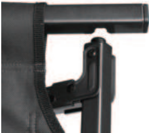
Step 4 Slide one end bar through the pocket at the foot of the cot. Make sure that the notch of the end bar is positioned as shown in figure 4. When positioned correctly, notch will fit over the button on the cot and can be pushed down to lock in place.
