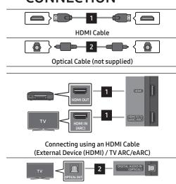
Connecting using an Optical Cable (D.IN)
