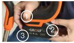
Step 1:Hold the machine Step 2:Press the battery button Step 3:Push the battery out
