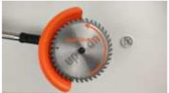
4:Screw on the backing plate screw. Please pay attention to the installation direction of the back plate screws.
