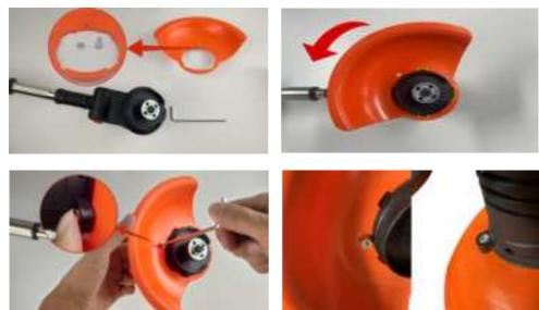
Remove the screws of the grass guard, and insert the grass guard into the machine head corresponding to the groove.
