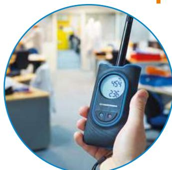
MISURARE LA TEMPERATURA DELL'ARIA AMBIENTE E L'UMIDITÀ RELATIVA (VENGONO CALCOLATI IL PUNTO DI RUGIADA E LA TEMPERATURA A BULBO UMIDO)
