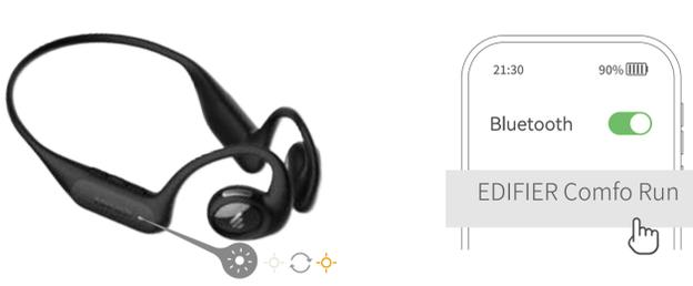
Power on and then select "EDIFIER Comfo Run" in your device setting to connect.
