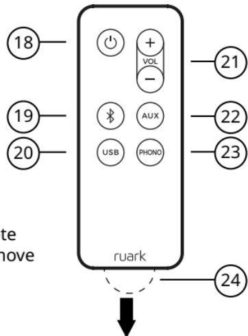
**Note:** Before using your remote for the first time you must remove the plastic battery tab (24) to activate the battery.
