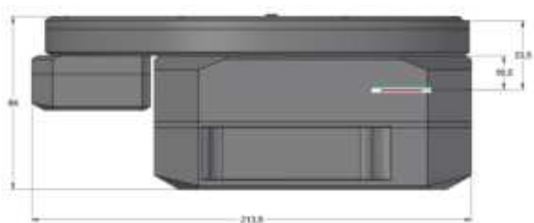
Figure 18: C3 camera head with External filter wheel side view dimensions
