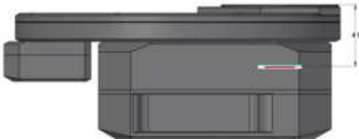
Figure 29: C3 camera with “M” External Filter Wheel back focal distances with M68 × 1 version 2 adapter
