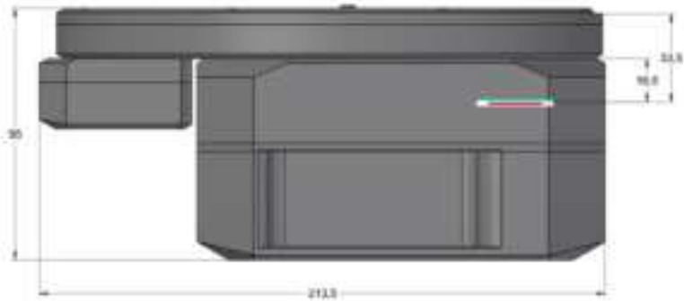
Figure 20: C3 camera head with Enhanced cooling and External filter wheel side view dimensions
