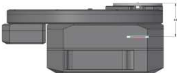
Figure 32: C3 camera with External filter wheel, the Canon EOS adapter is attached to adapter base on the External filter wheel
