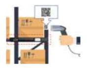
Each cell is assigned a unique QR code, and when it is scanned by the scanner, the unique QR code of the indicator to be newly registered is rescanned and automatically registered to the server.
