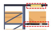
Attach it to each cell to use LED lights that work with the indicator to increase visibility of the operator to prevent job errors.
