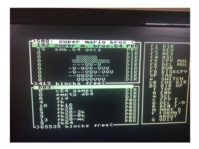
The leftward arrow key allows for switching between drives 8 and 9.
