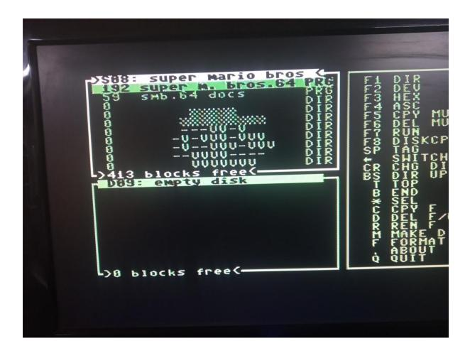
To start the process of copying, press the F8 key (SHIFT + F7).
