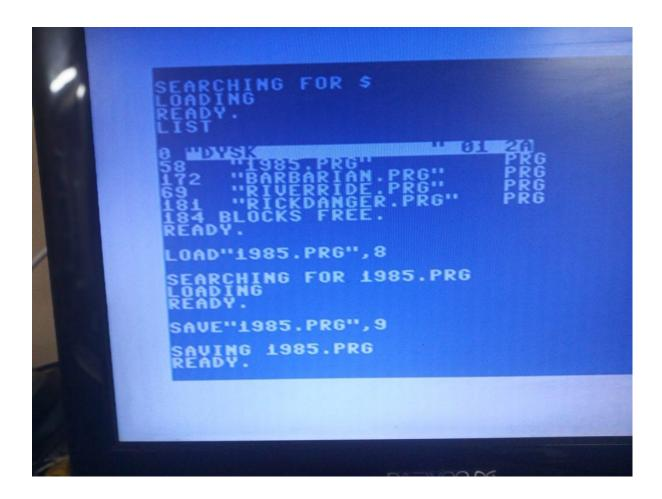
The picture above shows a game that has been loaded from disk drive number 8 to the computer memory, which was subsequently saved to a SD2IEC set as drive number 9.
