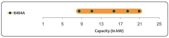
$Note: The above capacity data are at the following condition. Ambient temp. + 38 ^{\circ}C, evaporating temp. - 25 ^{\circ}C, return gas temp. + 18.3 ^{\circ}C, subcooling 2.8 KeV and the following condition of the follo$
