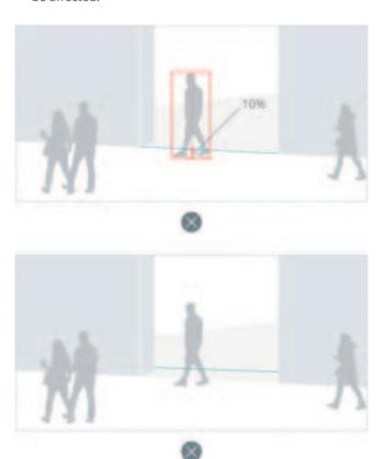
Place the detection fences in the middle of the screen and remove obstructions like potted plants or columns, so that objects can be properly detected on either side of the fences.
