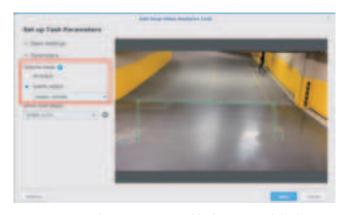
• **All objects**: This option is suitable for sites with higher alert levels as it includes all types of intrusions. Events will be triggered when 30% of the object areas cross the fence.
