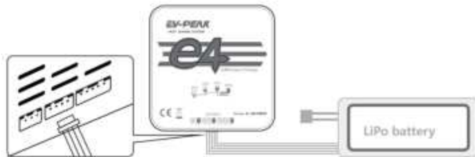
Figure 19: Cube Balance Charger Connection
