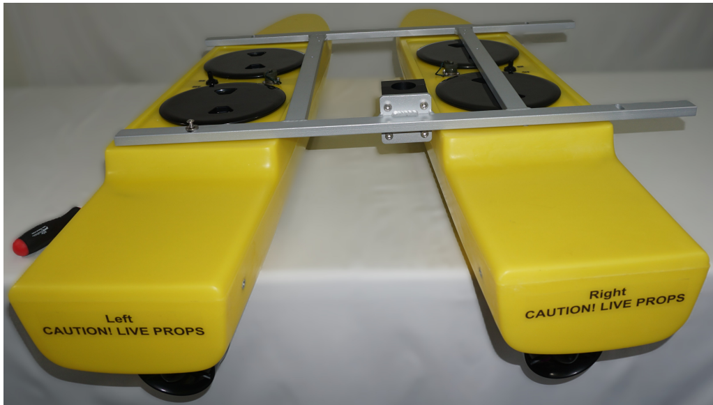
Figure 9: Pontoons Not Spaced Correctly
