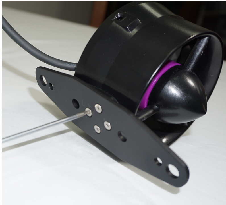
Figure 58: Thruster Adapter Plate Removal
