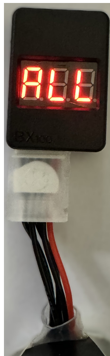
Figure 17: LiPo Voltage Tester
