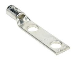
Penn-Union BLU series compression lug, standard barrel, tinplated copper, 35 kV, 1/2in mounting bolt, 2-hole, 1.75in hole spacing, 2/0 AWG, black markings.
