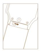
1. On the back of the strap, 2. Gently pull strap away slide the embedded lever to the right.
