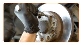
16 Remove the brake disc.
