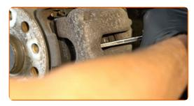
Remove the brake caliper. Use a crowbar.
