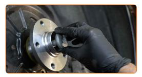
Tighten the hub. Use XZN #16. Use a torque wrench. Tighten it to 180 Nm torque.+180°
