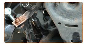
13 Remove the caliper bracket.
