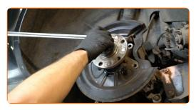
19 Remove the fastening bolt.
