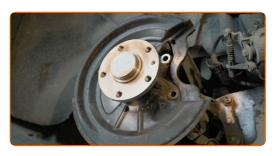
27 Install the brake disc.
