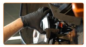
Tighten the brake caliper bracket. Use XZN #14. Use a torque wrench. Tighten it to 90 Nm torque.+90°
