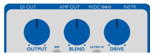
**9VDC:** Connect a 9VDC 2.1mm centre-negative mains power adaptor (minimum 150mA).
