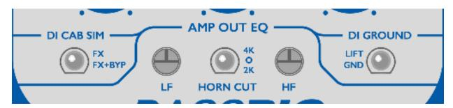
The post-drive AMP OUT EQ ensures compatibility with a wide range of amps and cabs. Instead of compromising your amp's tone controls to suit the BASSRIG, set your amp for your preferred clean sound then use the EQ controls to adjust the pedal's output accordingly (see tables on page 8).
