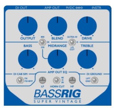
**DRIVE:** The gain control functions exactly like the volume knob on a non-master-volume valve amp. Turn it clockwise for more gain, drive and distortion. Turn counterclockwise to clean things up.
