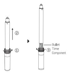
Tip: To retract the Bullet Time Component, loosen the knob and shorten the stick.
