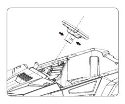
3.Install the wind deflector Insert the wind deflector into the specified position of the vehicle body.
