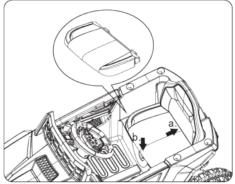
7.Mount the handrails Insert directly into both sides of the body as shown in the figure.
