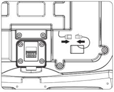
6.Install the backrest into the body and fix it with tw
