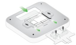
3. Slide the access point into the bracket until it locks in place. The locking tab must be at the front of the access point.
