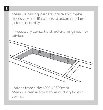
**Note:** The installer is to ensure that the framing is in accordance with NZS 3604:2011 or get specific design instructions from a suitably qualified engineer.
