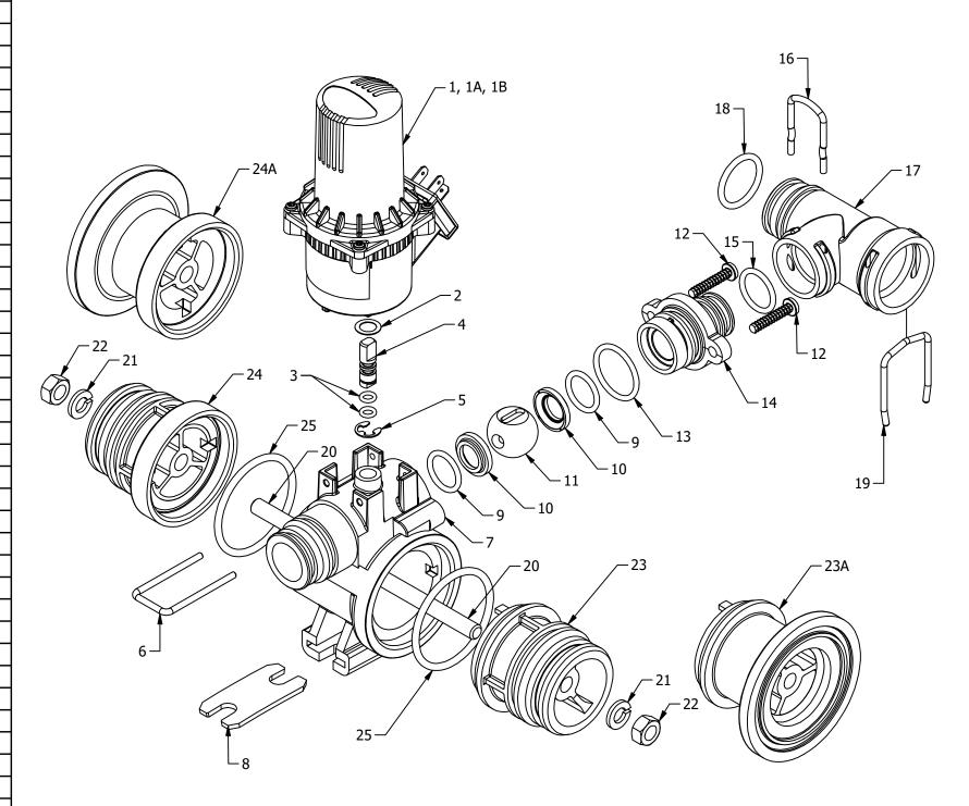
ASSEMBLY NOTE: WHEN ASSEMBLING THE MANIFOLD, CENTER THE CONNECTING ROD (ITEM 20) BEFORE TIGHTENING HEX NUTS (ITEM 22).
