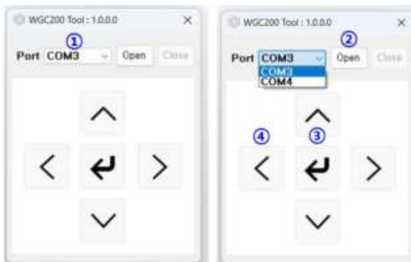
[FIG. 5.1.1] UART control Program
