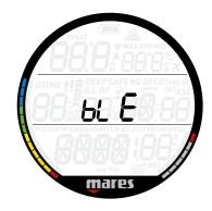
This submenu allows you to communicate with an external device via Bluetooth. Press and hold the button and the display will show **bLE SENd**, symbolizing that Puck Air 2 is ready to communicate.
