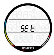
Puck Air 2's **SEt** menu allows you to change settings. Once inside this menu, press the button to scroll between two submenus: **SEt dIVE**, where you can set parameters pertaining to the dive, and **SEt tIME**, where you can set parameters pertaining to time and date.
