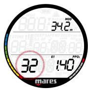
Once inside this menu, press the button to change the  $\mathrm{O_2}\%$  and observe how this affects the maximum operating depth [MOD]. Then press and hold the button to move on to the  $\mathrm{ppO_2}$ max and use the button to change the value, again noticing how this affects the MOD. Press and hold the button again to save the setting.
