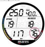
When the oxygen toxicity level reaches 100% the alarm is repeated for 5 seconds in one-minute intervals after the first occurrence and for as long as the value of CNS stays at or above 100%. Consider terminating the dive immediately!
