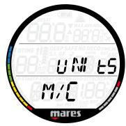
You can choose between metric (depth in meters, temperature in °C, tank pressure in bar) and imperial units. (depth in feet, temperature in °F, tank pressure in psi).
