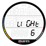
Puck Air 2 has a backlight which can be activated in case of low ambient light. The backlight is activated by pressing and holding the button. During a dive, the backlight will stay on for the duration defined in this menu. You can choose between 1 and 10 seconds.
