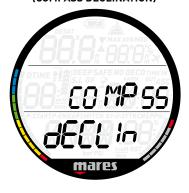
Depending on the exact location on the planet, there can be a deviation between true North and magnetic North. Any compass will always show magnetic North, so via this menu you can set a value for the so-called declination that will make the compass show true North instead.
