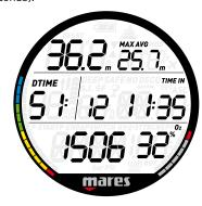
Press and hold the button to view the next page of the dive log, which shows the surface interval prior to the dive instead of the dive time, the tank pressure (alternating starting, ending and differential value every 2s) and CNS (alternating between start and end value) in the bottom row. Press and hold the button to return to the list of dives.
