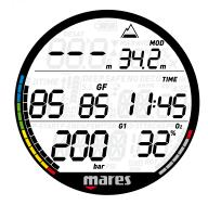
The pre-dive display shows the set gradient factors (alternating with the surface interval if there is remaining desaturation) and altitude class, time of day and tank pressure (when available). If Nitrox is set, it will show the  $\rm O_2$  percentage and the corresponding MOD.
