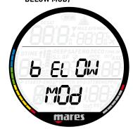
When set to **ON**, Puck Air 2 will allow a switch to a gas at a depth deeper than the MOD of the gas (resulting in an immediate MOD alarm).
