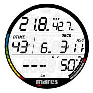
If you press the button (as opposed to pressing and holding it) while G2 is blinking, the next available gas in the list will be displayed instead. This will be G1 or G3 (if set), depending on the depth and whether you allowed the switch below MOD.
