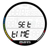
This menu allows you to set the time and date. Press and hold the button and **24h** or **AMPM** will start to blink. Press the button to switch between the two and/or press and hold the button to confirm and move on to set the hour, the minutes and the date.
