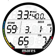
For **DECO** stops, since the duration is a function of the exact depth, only the minutes are shown.
