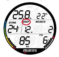
In a **DECO** dive, the depth of the deep stop replaces the depth of the deepest **DECO** stop. and the duration of the stop is not shown to avoid misinterpreting it as a **DECO** stop.
