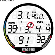
In this case, if the diver attempts a repetitive dive after surfacing, Puck Air 2 will function only as a depth gauge and timer (bottom timer mode), and it will display on the screen.
