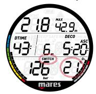
Press the button while this indication is blinking to initiate the gas switch: the oxygen percentage of G2 starts to blink in lieu of that of G1, and in the top right corner the MOD of G2 is displayed, also blinking.
