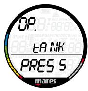
The third menu, **tANK WARN**, is the value at which Puck Air 2 triggers a half tank warning **(G1** only). Default values are **100bar** and **1500 psi**.
