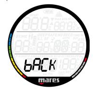
During the dive, press the button to access alternate information on the display and press and hold the button to activate the backlight, the compass or to initiate the gas switch sequence (described in 3.6 and 3.8, respectively).
