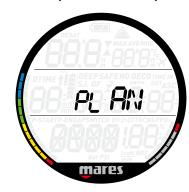
This function allows you to plan your next dive. Upon entering this menu, the middle row shows a surface interval of 0:00: in case you dived recently, you can enter an additional surface interval in 15-minute increments between now and when you intend to dive by pushing the button; the residual nitrogen load will be adapted accordingly. Next press and hold the button to enter the actual dive plan: Puck Air 2 displays a depth and the corresponding no deco time.
