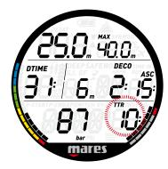
Additionally, when the tank pressure reaches the value specified under **tANK RSRV**, the tank pressure starts to blink and an audible alarm goes off. Press the button to acknowledge the alarm and silence it, though the tank pressure will continue to blink.
