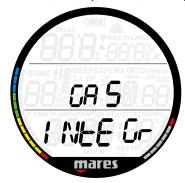
This menu contains four submenus. The first menu, tANK VOLM, allows you to set the size of the volume of the tank (G1 only). This parameter is important for a correct evaluation of your gas consumption in l/min or cu ft /min. Default setting is 12l for metric system and 80 cubic feet in imperial. For the imperial setting it is paramount that you also set the correct operating tank pressure, since the size of the tank is referenced to this pressure.
