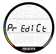
When set to **ON**, Puck Air 2 will consider all set gases in the decompression calculation, with switches carried out at the MOD of each gas. When set to **OFF**, the decompression calculation will consider the currently breathed gas only. See Section 3.8 for more information about the **PrEdICt** feature.
