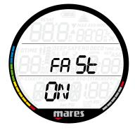
If the ascent rate exceeds 120% of the allowed value over a depth change of more than 20m/66ft, due to the potential of harmful bubble formation, Puck Air 2 locks the computer for 24 hours in order to prevent you from diving again. In this menu, you have the option to disable the locking up of the computer in the event of an uncontrolled ascent.
