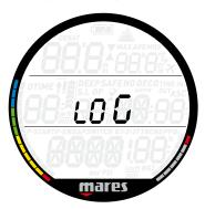
Puck Air 2 can record the profiles of approximately 150 hours of diving, at a sampling rate of 5 seconds. The information can be transferred via Bluetooth to an external device. In addition, Puck Air 2 can show most of the information directly on the display.
