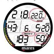
Press and hold the button to confirm the switch to G2: the set oxygen concentration will be displayed steadily in the lower right corner of the screen: if **PrEdICt** is set to **ON**, the decompression calculation will not change; if **PrEdICt** is set to **OFF**, within 20 seconds of having switched gas, the decompression calculation will be updated to reflect the change in gas. In addition, the tank pressure will show ----
