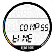
You may use the compass for long stretches of navigation or you may just glance at it once in a while to get a bearing. In the latter case you may want the display to automatically return to the regular display after a set number of seconds. The default value is **ON**, meaning that you return to the regular display by pressing or pressing and holding the button, but you can set it to 5, 15, 30 or 60 seconds.
