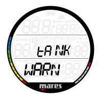
The fourth menu, **tANK RSRV**, is the value at which an alarm is triggered because you should always be at the surface before reaching this level. Furthermore, this value is used to calculate the **TTR** value (see section 3.3.5 and 3.4). Default values are **50bar** and **500psi**.
