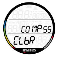
The digital compass in Puck Air 2 is calibrated from the factory and does not require, under normal circumstances, any further maintenance. In certain instances, however, such as after exposure to extremely intense magnetic fields, it may be necessary to recalibrate the compass to ensure its accuracy. If you notice an obvious deviation in the indication of the compass, access this menu and perform the calibration as described below.
