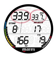
The alarm persists until the diver has ascended enough for the  $ppO_2$  to return within the set limit.
