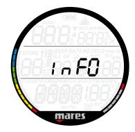
This submenu provides information about the hardware and software of your Puck Air 2 and about the status of the battery: **OK** means the battery is good, **LOW** means the battery is weak but you can still do a few more dives, and **KO** means the battery is very low and Puck Air 2 won't function as a dive computer.
