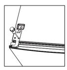
9. Take left hinge cover from accessary bag and install it with top hinge. Then install hole cover at right side.
