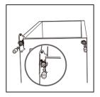
7. Make the middle hinge reverse the direction 180°C, then transfer it to the left property position. Make the middle hinge pin in the upper hole of the lower door, then tight the screws.
