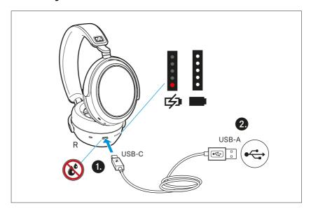
Make sure that the charging socket is free from moisture and contamination. Connect the USB-C connector of the charging cable to the USB socket of the headphones.
