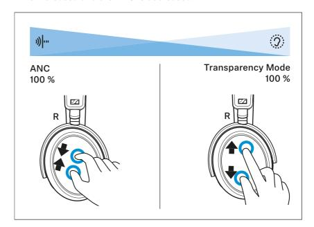
You can also adjust the intensity of the active noise cancellation ANC and the Transparency Mode via a slider in the Smart Control app.
