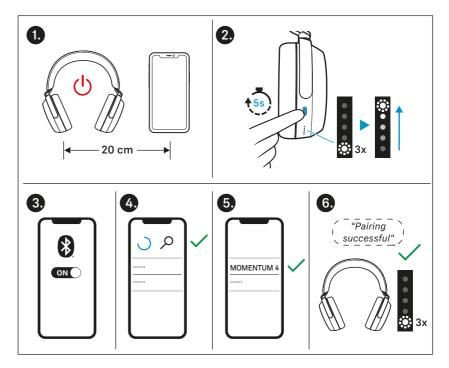
If no connection is established within 2 minutes, pairing mode is terminated and the headphones switch to standby mode. If necessary, repeat the steps described above.
