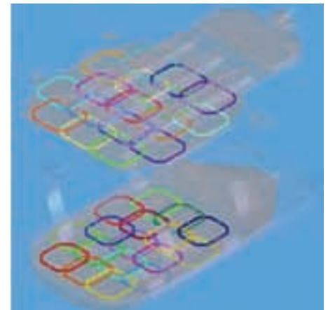
Figure 2. Element orientation of anterior and posterior sections of 32-channel torso coil.
