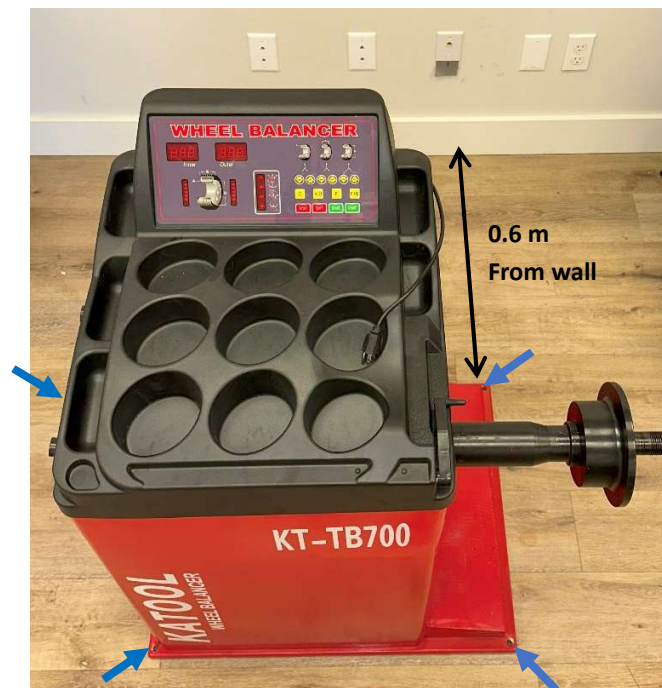
Figure 2.0 – Always lift the machine upright evenly from the front and back (See the red arrows)
