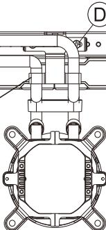
It is possible to adjust the position of the screw based on the case to control the water pipe fastener so that it is right above the CPU./
