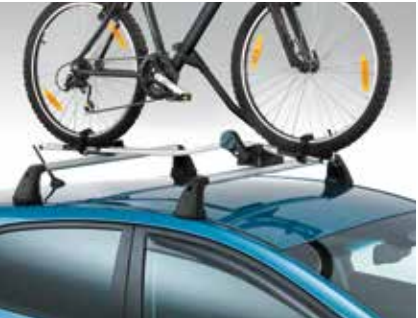
ProRide 591 bike carrier. After the bike is placed upon the frame holder, all adjustment and securing can be carried out at roof height using the single-handed rotary knob. The weight limit is 20 kg. 55701SBA10 (5dr + 3dr + Wagon)
