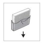
Before using the air purifier for the first time, open the purifier panel and remove the composite filter. Make sure to remove any packaging from the filter element, or the product will not function correctly.
