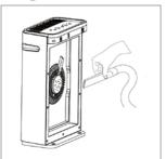
Clean out any remaining dust, dirt, or hair inside the purifier using a vacuum hose or dry cloth.
