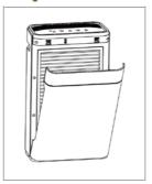
Place the new filter into the air purifier making sure it is the correct way around. The black side of the filter should be on the inside, closest to the fan. Airflow travels from outside to the center of the unit. Refit the purifiers panel, and plug the power cord back into an electrical outlet.
