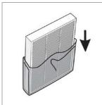
**Important!** Remove any packing from the new filter element. Take notice that one side of the filter is black in color; this side needs to be facing inwards.
