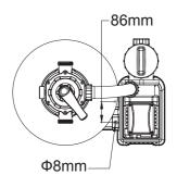
3. EN60335-2-41 TEST standard requires the sand filter to be vertically fixed on ground or a certain pedestal made of wood or concrete before use to prevent the sand filter from accidentally falling. Fully assembled sand filter will exceed 18kg. The mounting holes should be 8mm in diameter and spaced 86mm apart. Use two bolts and nuts with a maximum of 8mm in diameter to fasten the sand filter to the pedestal.
