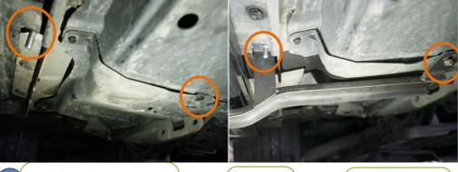
Middle Bracket: Remove 2 clips which are at the middle side of the car chaais. Find a hole hidden inside the guard plate.Cut out a small hole to
