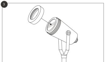
Keeping the silicone gasket on the glass lens, replace the lens on top of the spring and screw the collar back on.
