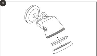
Once the bulb is connected, replace the glass lens with the thicker side of the rubber gasket facing the bulb.
