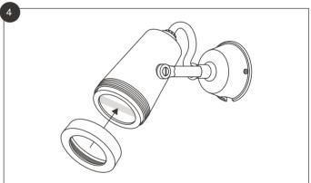
Keeping the silicone gasket on the glass lens, replace the lens and screw the collar back on.
