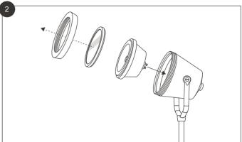
Unscrew the brass collar to remove the glass lens. Insert the
