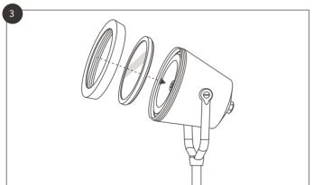
Once the bulb is installed, replace the glass lens, making sure the thicker side of the rubber gasket faces the bulb. Then screw the brass collar back into place.
