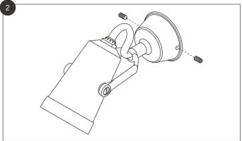
Place the light body over the mounting bracket and use the grub screws provided to fix it in place.
