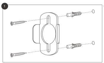
Drill two 6mm holes, set the anchors, and screw the mounting bracket to the wall using the screws provided. Consult a qualified electrician to connect the light to the mains power.
