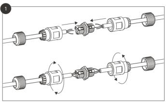
Connect the wires using the waterproof terminal.
