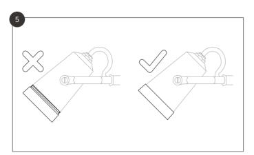
Important: make sure the brass collar is tightened all the way, as this is necessary for the IP rating of the light.
