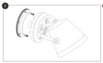
Use the grub screws provided to attach the light to the mounting ring.
