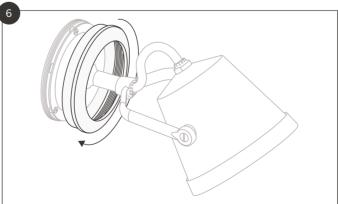
Screw the ring onto the mounting base.
