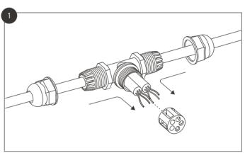
Connect the wires using the waterproof terminal.
