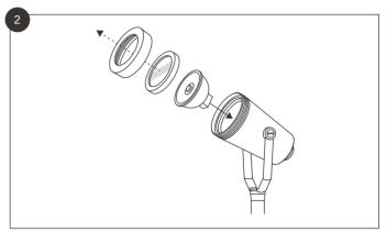
Unscrew the brass collar to remove the glass lens and spring. Insert the bulb.
