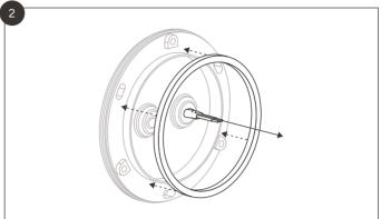
Put the grommet back in its place and push the wires through it. Make sure the gasket is attached to the mounting base.
