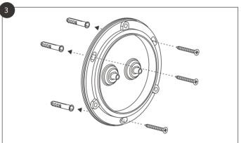
Drill three 6mm holes and set the anchors to attach the mounting base to the wall.
