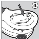
4. Insert the new battery, negative end first, as shown in Figure 3. Ensure that the polarity is correct (align the positive end '+' of the battery with the '+' symbol in the battery housing). Replace the Battery Cover and ensure that it is correctly closed (Figure 4).
