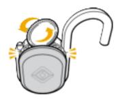
5. Carefully remove the cover to avoid damaging the tabs.
