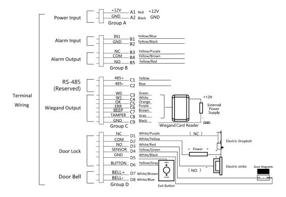
Note: The external power supply and the access control terminal should use the same GND cable.
