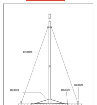
**DYA019**Foldable system for mast Ø 50 mm
