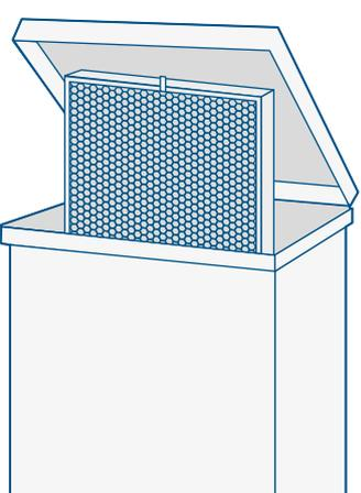
Remove pre-filters and main filters, and dispose of them (both sides).
