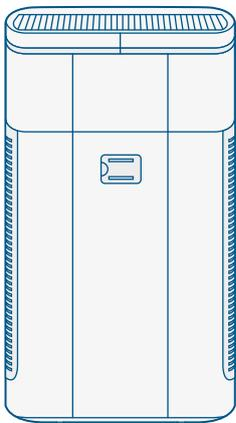
To clean the particle sensor (back of Rediair) lift flap and carefully clean with a cotton swab. This should be done every 2 months or if the LED air indicator consistently shows poor air quality.
