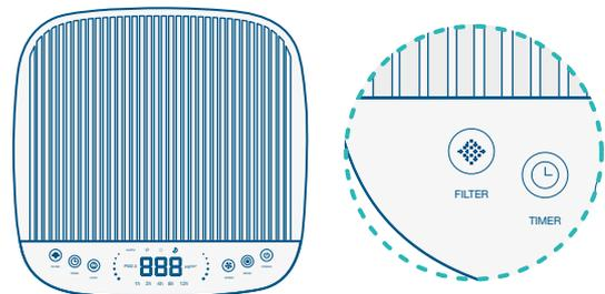
To re-set the pre-filter timer, hold the filter button for 5 seconds until it beeps
