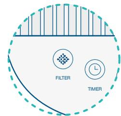
To reset the timer after changing the filters, press and hold the filter indicator for 5 seconds until it beeps, at which point the filter light will stop flashing
