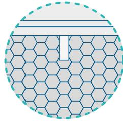
Install the new main filters (both sides), making sure that the tabs are facing outwards.
