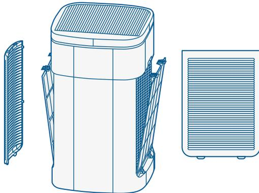
Re-install the external covers and the pre-filters (both sides). **Note:** Ensure external covers are fitted correctly or the Rediair will not power-on.
