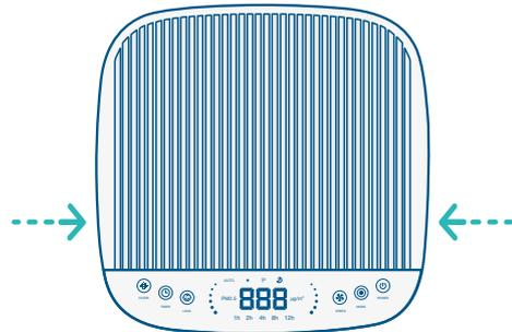
To clean Rediair's air outlet, lift the grill from the recesses indicated by the arrow symbols and clean the area with a dust cloth.
