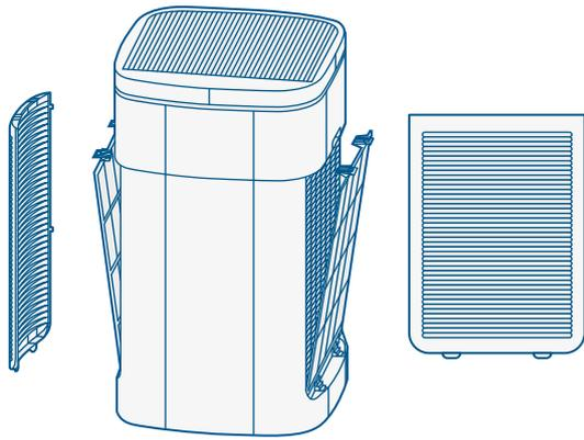
Remove the external covers and the pre-filters (both sides).
