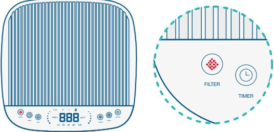
When the filter indicator (on the LCD touch control panel) lights up continuously red OR flashes 5 times and then turns **continuously red** for 5-seconds, it is time to change the all filters.
