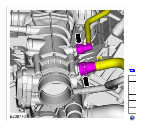
Disconnect the hose couplings at turbocharger inlet tube.
