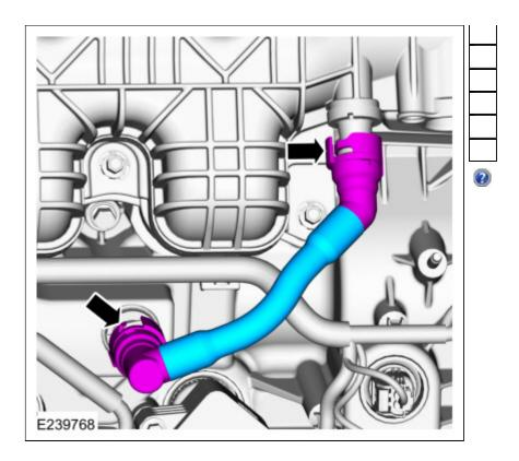
7. Disconnect the wire harness retainers from the intake manifold.
