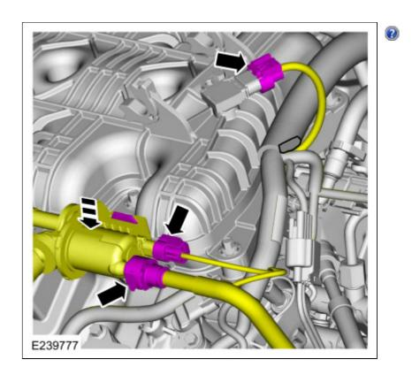
Connect the quick connect couplings at turbocharger inlet tube.
