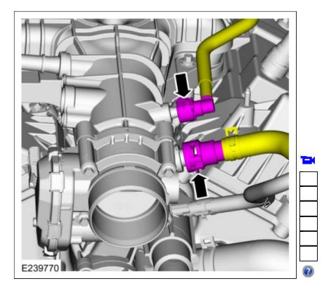
6. Connect the wire harness retainers to the intake manifold.
