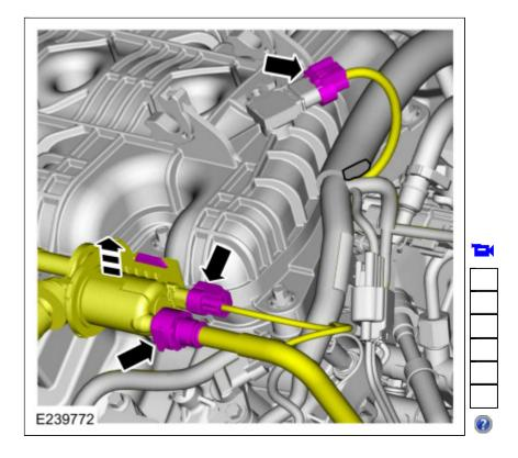
11. Remove the bolts and the intake manifold.
