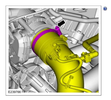
5. Disconnect the throttle body electrical connector and wiring harness retainer.
