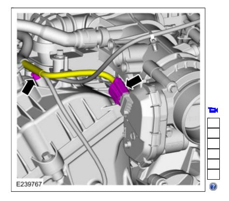
9. Position back the throttle body intake pipe and tighten the clamp. *Torque*: 44 lb.in (5 Nm)
