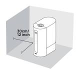
S Place the humidifer on a flat, level surface, keeping at least 30 cm / 12 inch away from walls or any major obstacles.
