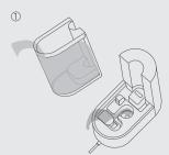
Drain any remaining water from the tank and the base.
