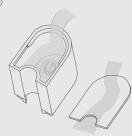
Remove the tank and detach the cover, drain any remaining solution from the tank and the base. Rinse the tank with water until the bleach smell is gone.
