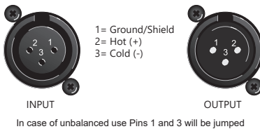
Balanced use of XLR connectors
