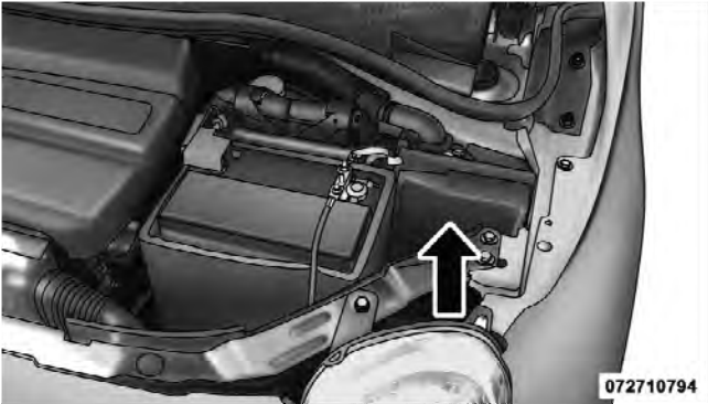
Front Distribution Unit
