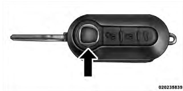
Remote Keyless Entry Transmitter With Mechanical Key Release Button
