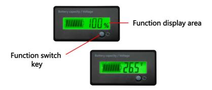
Continuously pressing the function key can cycle between voltage, battery percentage, and on/off screen switching
