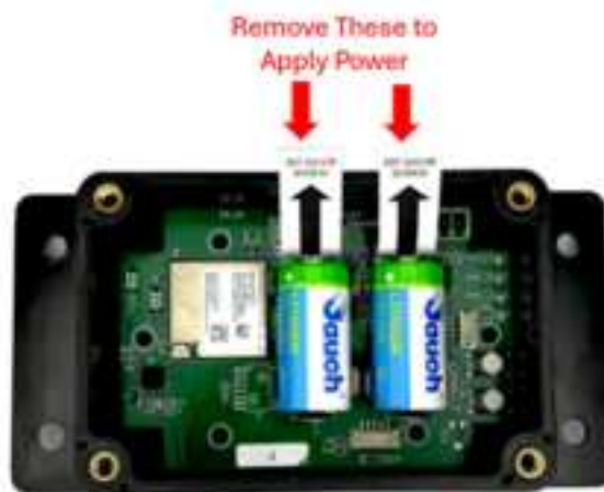
Picture 3: Battery Insulating Pull Tabs. Remove to Apply Power.
